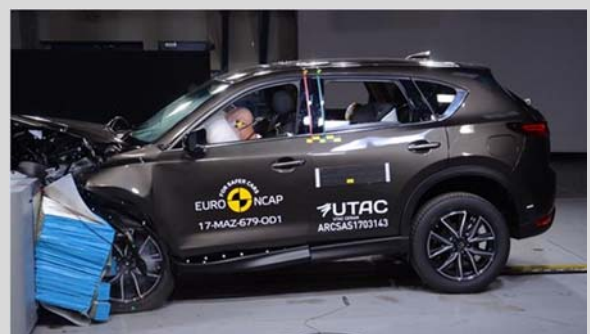
Frontal offset test at 64km/h
